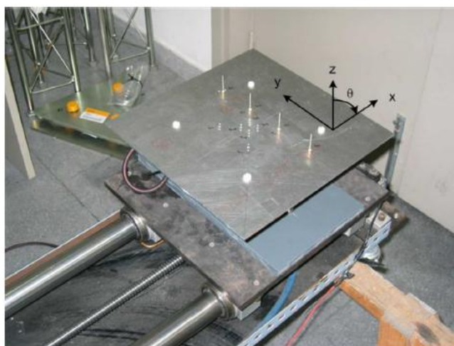
Fig. 1. Picture of the multiomnidirectional-beam MEA consisting of a ULA of omnidirectional monopoles over a finite ground plane, mounted on the automated measurement setup.
